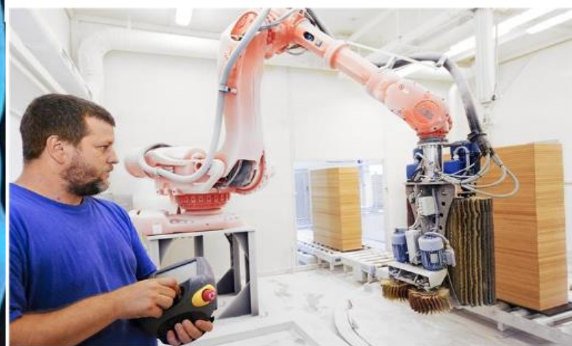
ABB IRB 6650 robots used for sanding the edges of panels before staining and painting
